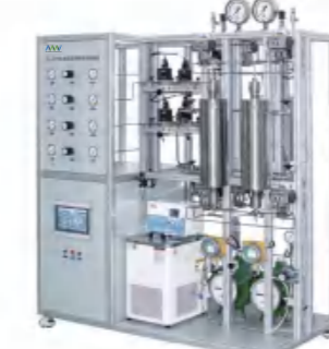
N 2 -O 2 pressure swing adsorption and desorption device
